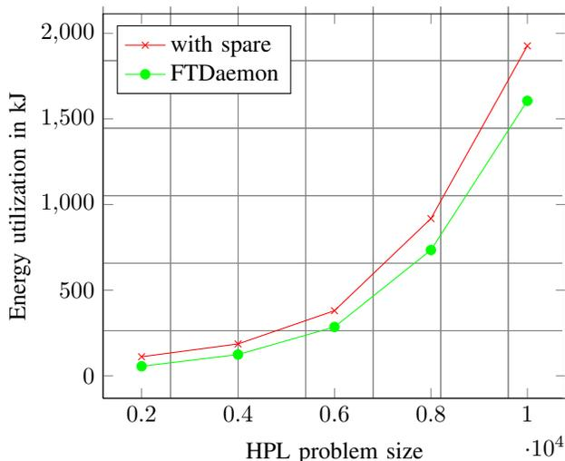
Figure 5: Energy utilization of FT with spare node compared with FTDaemon.
