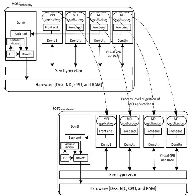
Figure 3. Fundamental architecture of our proposed solution
