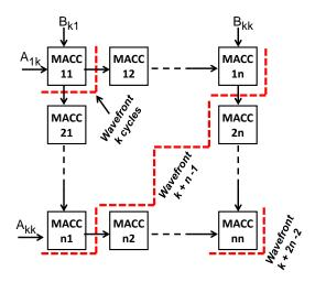
Figure 6. Wavefront systolic array operation.
