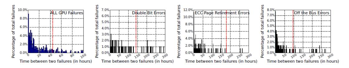
Figure 5: GPU failures exhibit temporal locality: These figures show the failure arrival time distribution. The dashed vertical line indicates the "observed" mean time between failure (MTBF). Multiple failures that occur beyond the x-axis limits are not shown here for clarity, but they contribute toward the MTBF calculation. Note that the combined MTBF is less than the MTBF for each individual types of failure.
