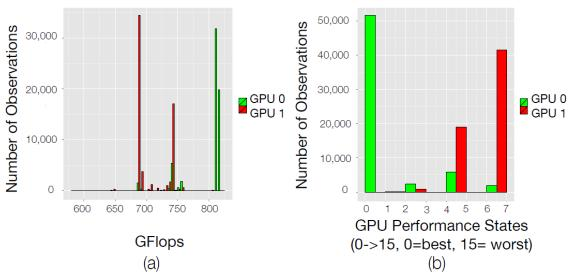
with two M2090 GPU cards: histogram of observed GFlops (a), histogram of observed performance-states (b).
