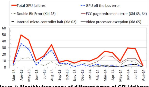
Figure 4: Monthly frequency of different types of GPU failures For the Titan supercomputer
