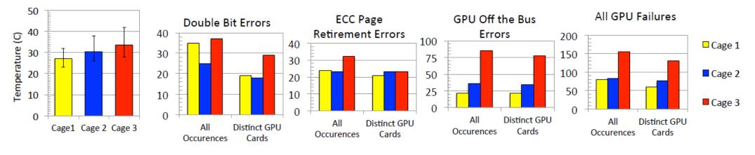
Figure 10: Temperature sensitivity of different GPU failures. Some GPU failure types tend to occur more in relatively hotter cages. "All Occurrences" counts all errors occurring in the same cage. However, in some cases, a single GPU card may see multiple errors. "Distinct GPU Cards" does not count repetitions of an error on the same card.
