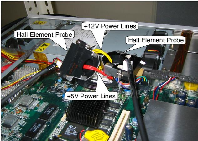
**Figure 8. Power Measurement using Hall Element Probes**
